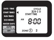
When you have set all desired START TIMES, press the MENU BUTTON to move to RUN TIMES.
